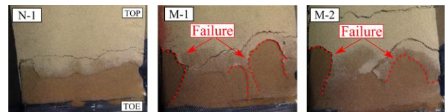
Figure 14. Deformation of embankment slope at land side after seepage test (Ikami et al. 2017)
