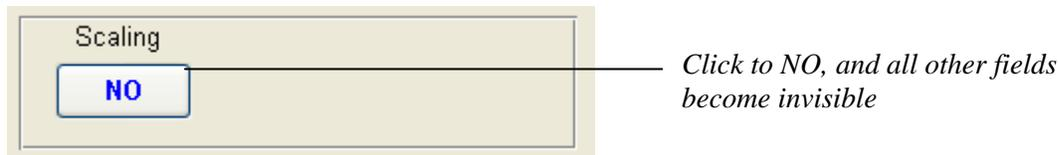
Click *Scaling* button to turn off scaling method. Original records are used in this case.
