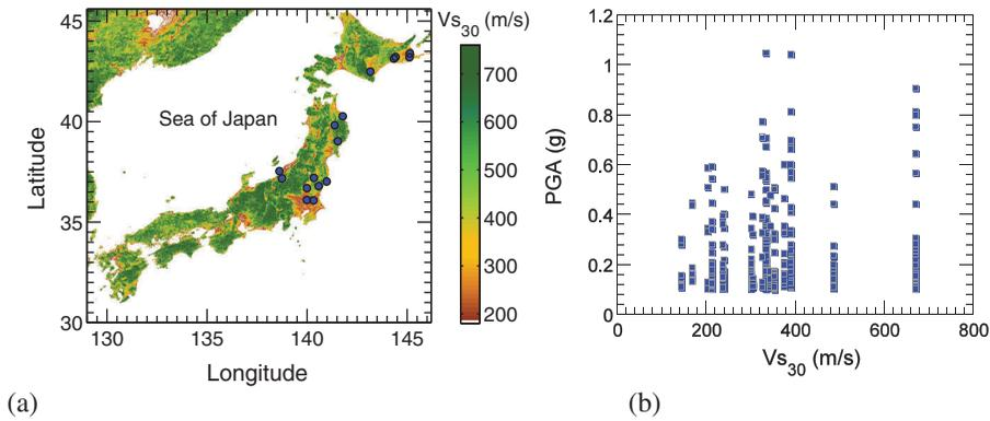
**Figure 9.** (a) Location of 16 strong-motion stations adopted in this study; (b) distribution of surface PGA versus  $V_{s30}$  for the 383 selected records used in this study.
