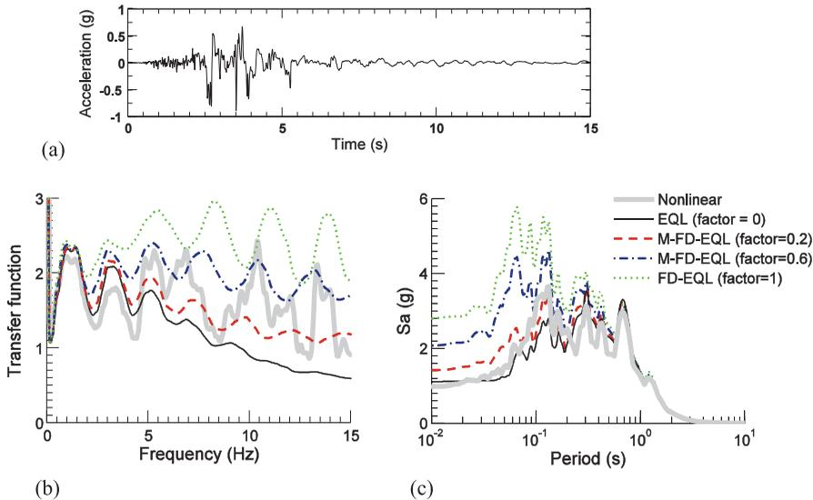
**Figure 4.** (a) Acceleration time history recorded at the Cerro Prieto station during the 1987 M5.5 Baja California earthquake as an input motion (b) Spectral accelerations and (c) transfer functions of ground response of a NEHRP class C site by the modified M-FD-EQL method (black line) and a fully nonlinear method (gray line) using the input motion.
