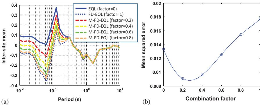
Figure 12. (a) Inter-site mean (fixed bias); (b) MSE for different combination factors.
