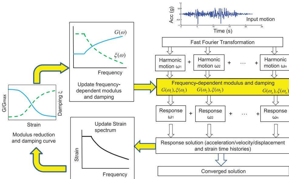
Figure 2. A flow chart of the frequency-dependent equivalent linear (FD-EQL) site response computation techniques.
