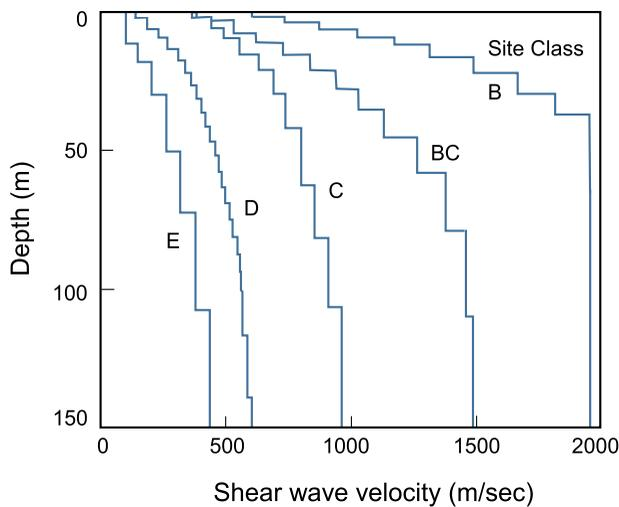
**Figure 5.** Average shear wave velocity profiles for generic NEHRP sites [adapted from Hartzell *et al.*, 2004].
