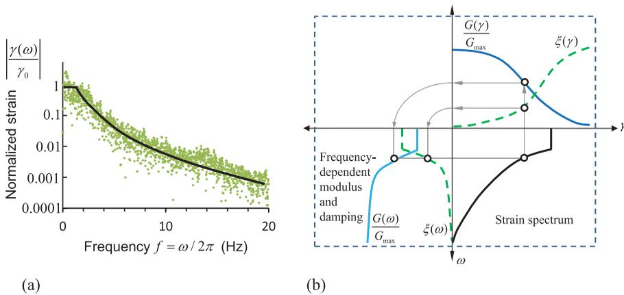
**Figure 1.** (a) An example of strain spectrum ( $\alpha = 0.12$  and  $\beta = 2.2$ , dots are discrete data of the strain spectrum, the solid line is a smoothed fitting function); (b) schematic of the evaluation of frequency-dependent material parameters [adapted from Kausel and Assimaki, 2002].
