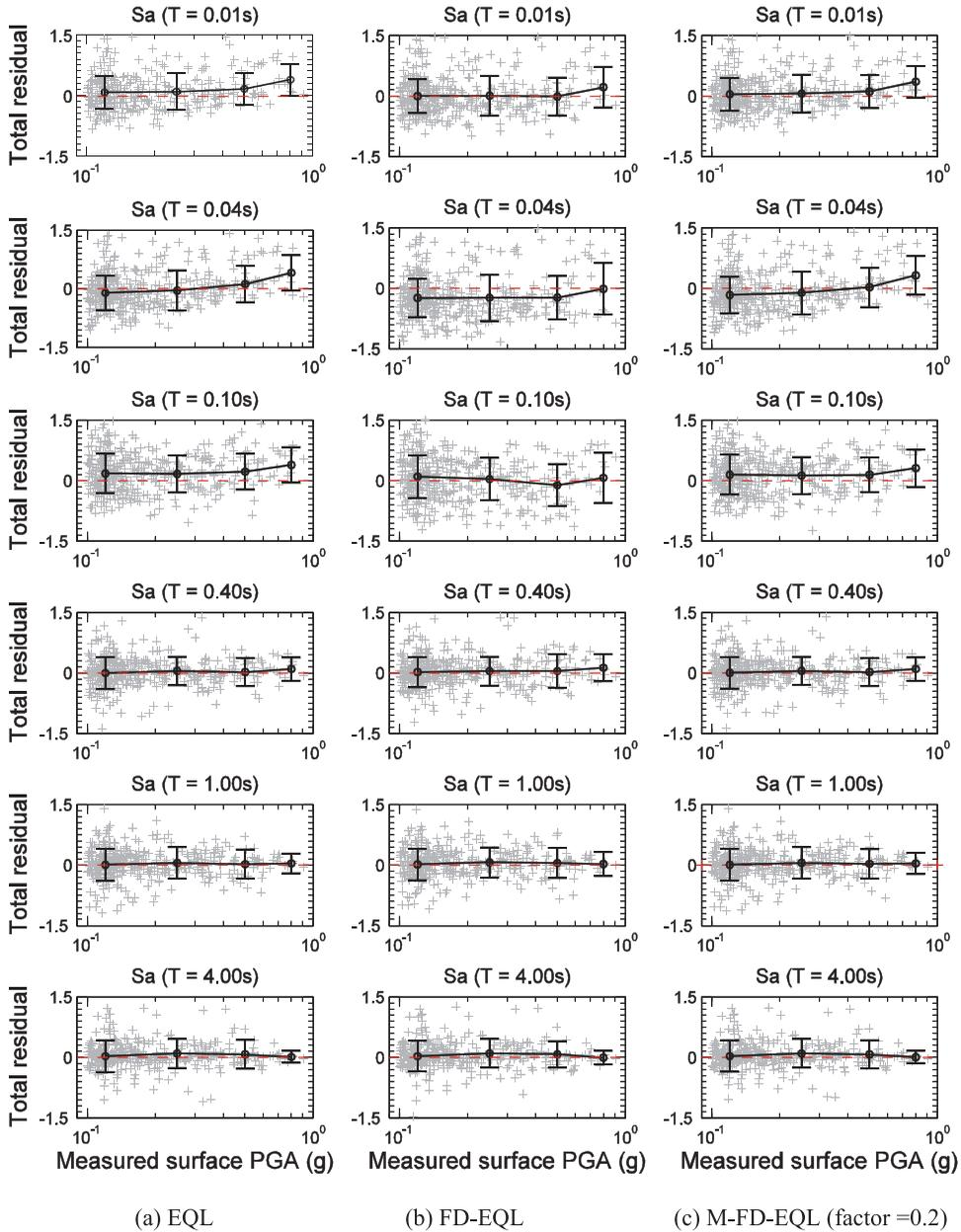
**Figure 10.** Total residual of ground responses for different spectra periods using the (a) EQL method, (b) FD-EQL method, and (c) M-FD-EQL method (factor = 0.2).
