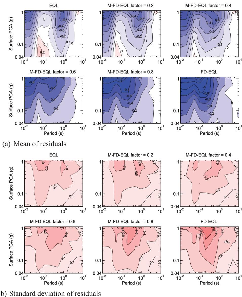
**Figure 8.** Contours of (a) mean and (b) standard deviation of residuals on NEHRP site class E.
