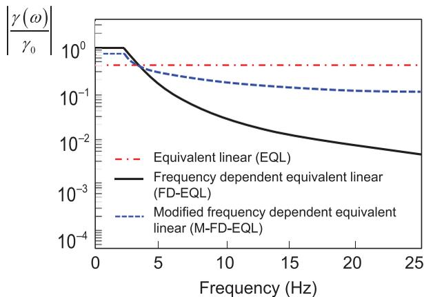
**Figure 3.** Strain spectra for the equivalent linear (EQL), frequency-dependent equivalent linear (FD-EQL) and modified frequency-dependent equivalent linear methods (M-FD-EQL).
