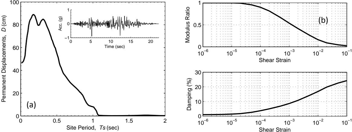
**Figure 1.** (a) Computed Permanent Displacements ( $K_y=0.1$  g). Insert: Acceleration Time History; (b) Modulus Ratio and Damping Curve for Nonlinear Soils.
