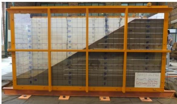
Figure 2. Constructed soil slope and plaster-strips in model 2
